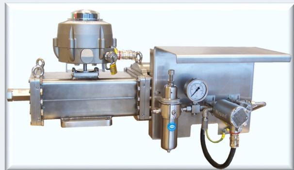
Quarter turn actuator with SDCU-20, local PST pushbutton and control panel
