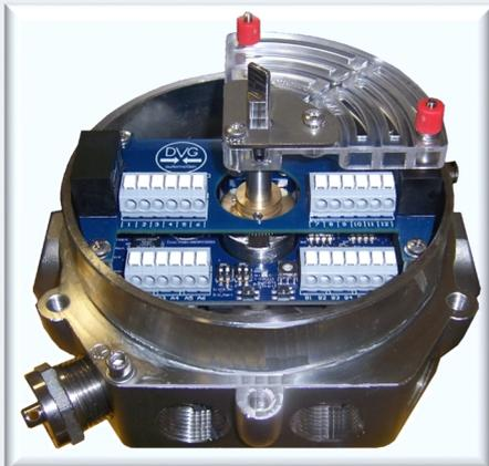
**SDCU-20 equipped with SDCU-20 LS and PST pushbutton**
