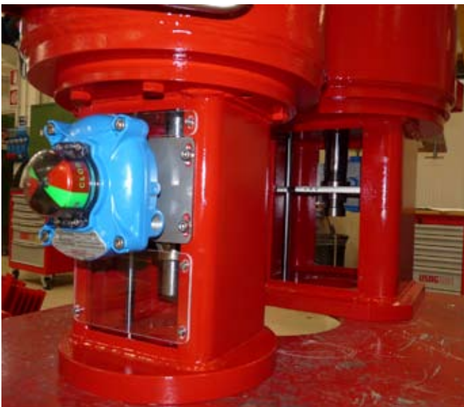
• Position transmitter with antirotation device
