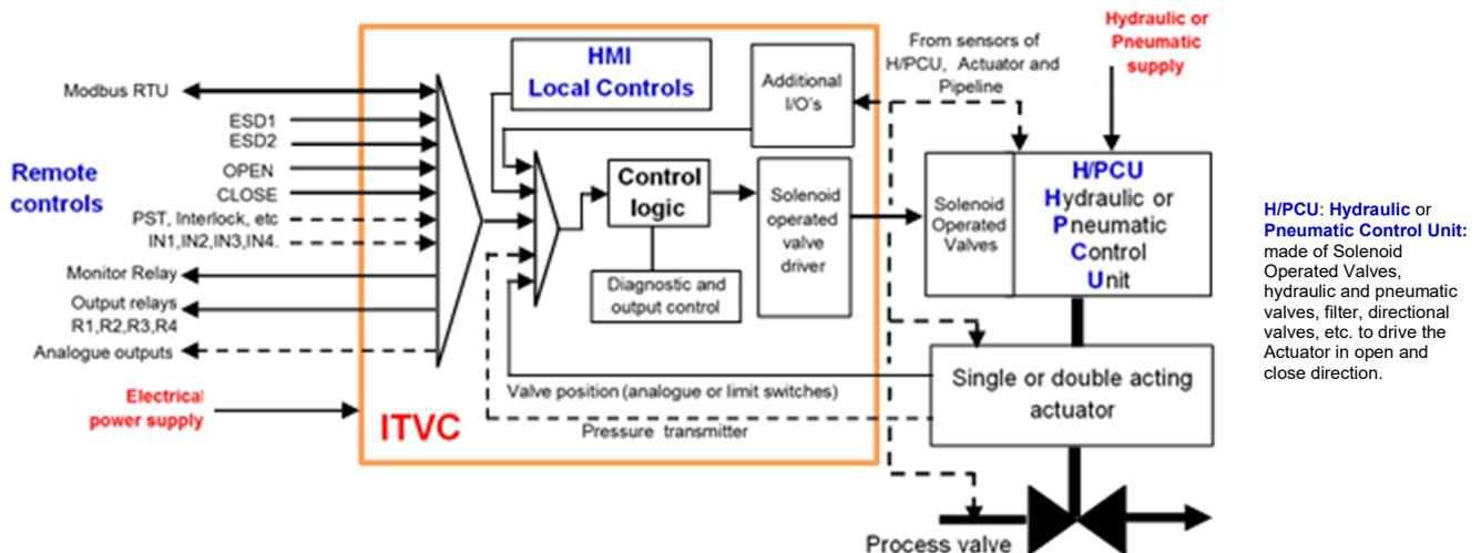
The ITVC collects the **commands** from control room and HMI, the **feedback sensors** signals from H/PCU, Actuator and Pipeline and **drives the Solenoid Operated Valves** of the **H/PCU** (Hydraulic or Pneumatic Control Unit) to **open and close the process valve** by means of the single or double acting **actuator**. Three actuator control mode are available: **LOCAL**, **REMOTE** and **OFF**. On request the **OFF** option can be removed.
