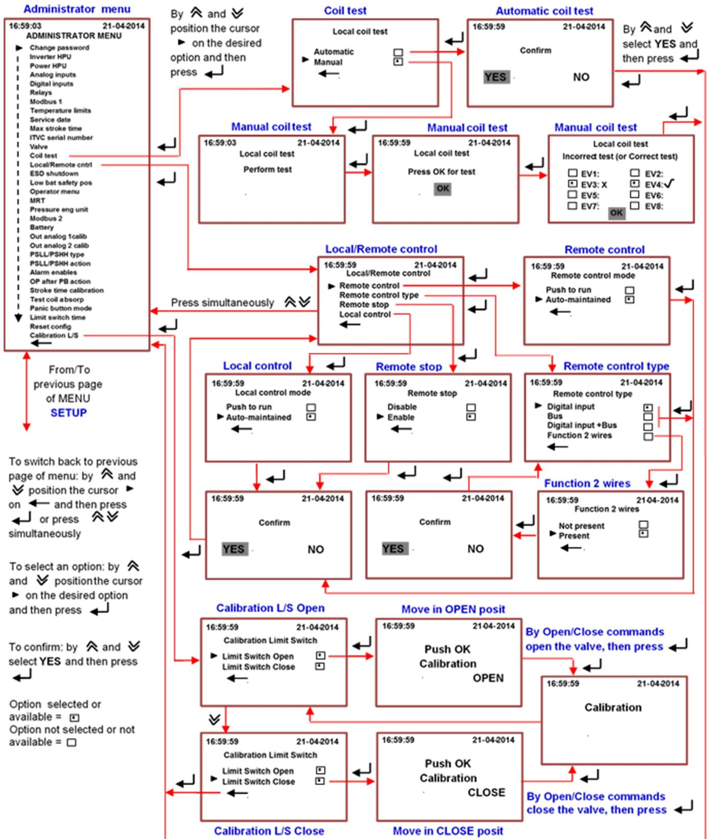
The following figure shows the procedure to set **ESD shutdown**, **MRT** and **Operator** menu
