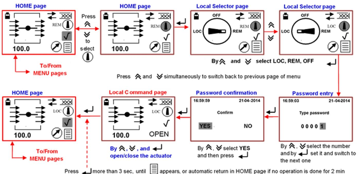
The same procedure can be used to switch from **LOCAL** or **OFF** to **REMOTE**. When the **Local Command** page appears, press
